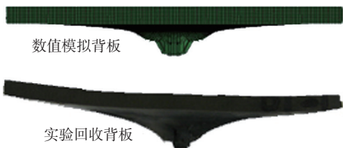
图2 数值模拟与试验结果背板最终形貌对比图 Fig.2 Comparison of simulation result and test result
